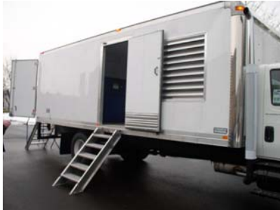
Vent for the Generator Room and The Door to the Control Room
